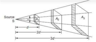
Let, 'S' be a point source of luminous intensity 'I' candela, the luminous flux emitting from source crossing the three parallel plates having areas A A, and A square meters, which are separated by a distances of d, 2d, and 3d from the point source respectively as shown in Fig.
