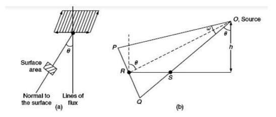
Let us assume that the surface is inclined at an angle ' $\theta$ ' to the lines of flux as shown in Fig. (a)
