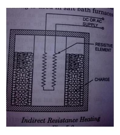
This arrangement provides a uniform temperature control can be provided in this case by presetting the time duration.
