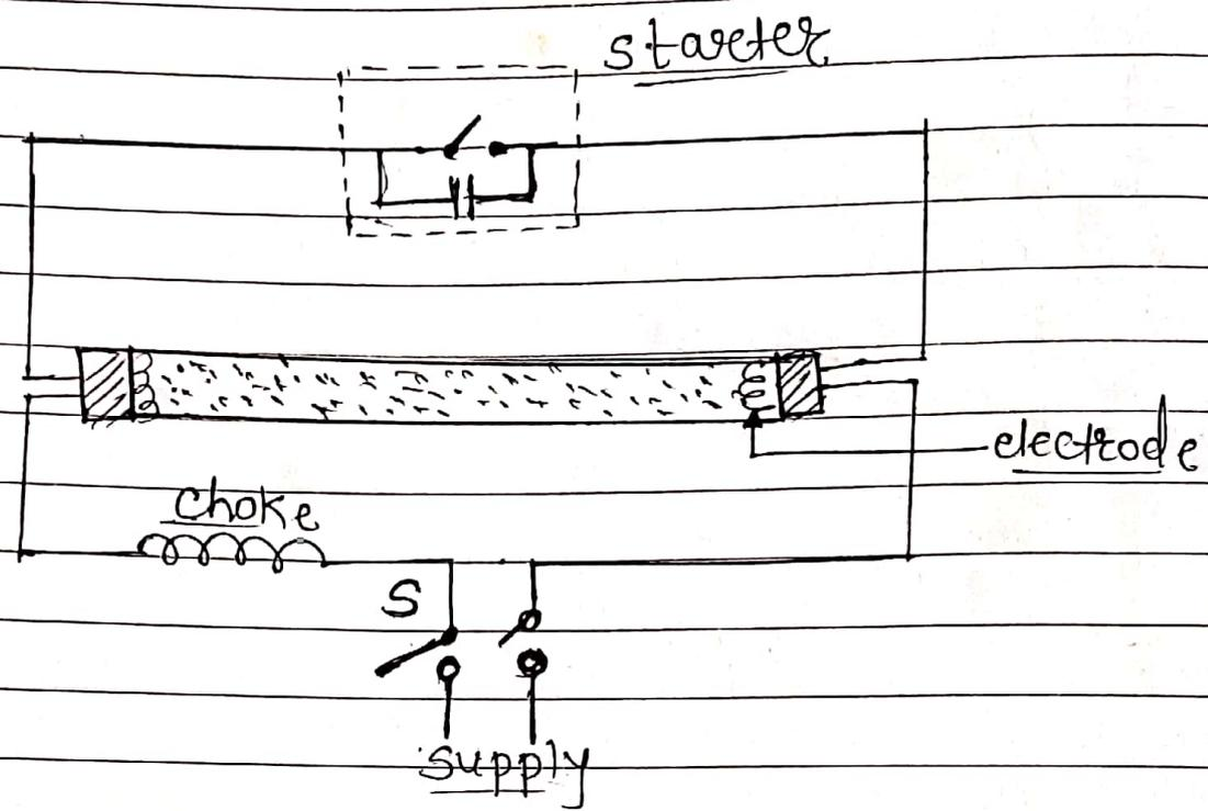
It consists of a long cylindrical tube. on the either side of the tube, two tungsten filaments are placed. the tube is coated with fluorescent powder from inside. and its filled with argon gas with small quantity of mercury. the control circuit consist of choke and starter
