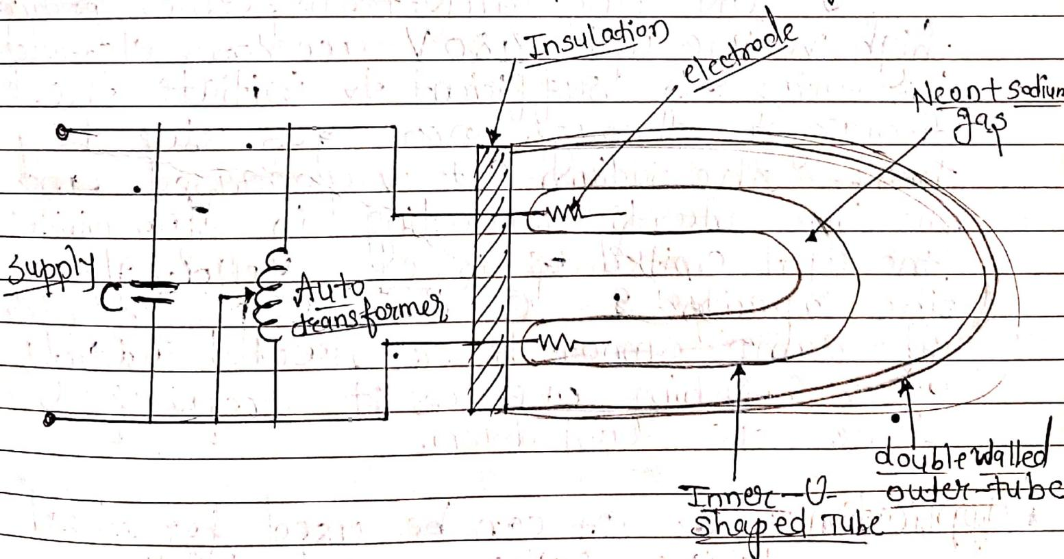
• Construction:- It consists of an inner-tube of U-shaped, and made up of a special Sodium-vapour resisting glass. It consists of two coated tungsten electrodes which are connected across an Auto transformer. The inner-U-tube contains neon gas and small amount of sodium. The inner-U-tube is enclosed in double walled vacuum flask type tube and is well insulated in order to conserve the heat required to vapourize sodium.
