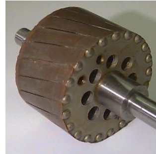
Fig 5. Squirrel cage rotor
