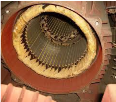
Fig.4 Stator with ribbed yoke
